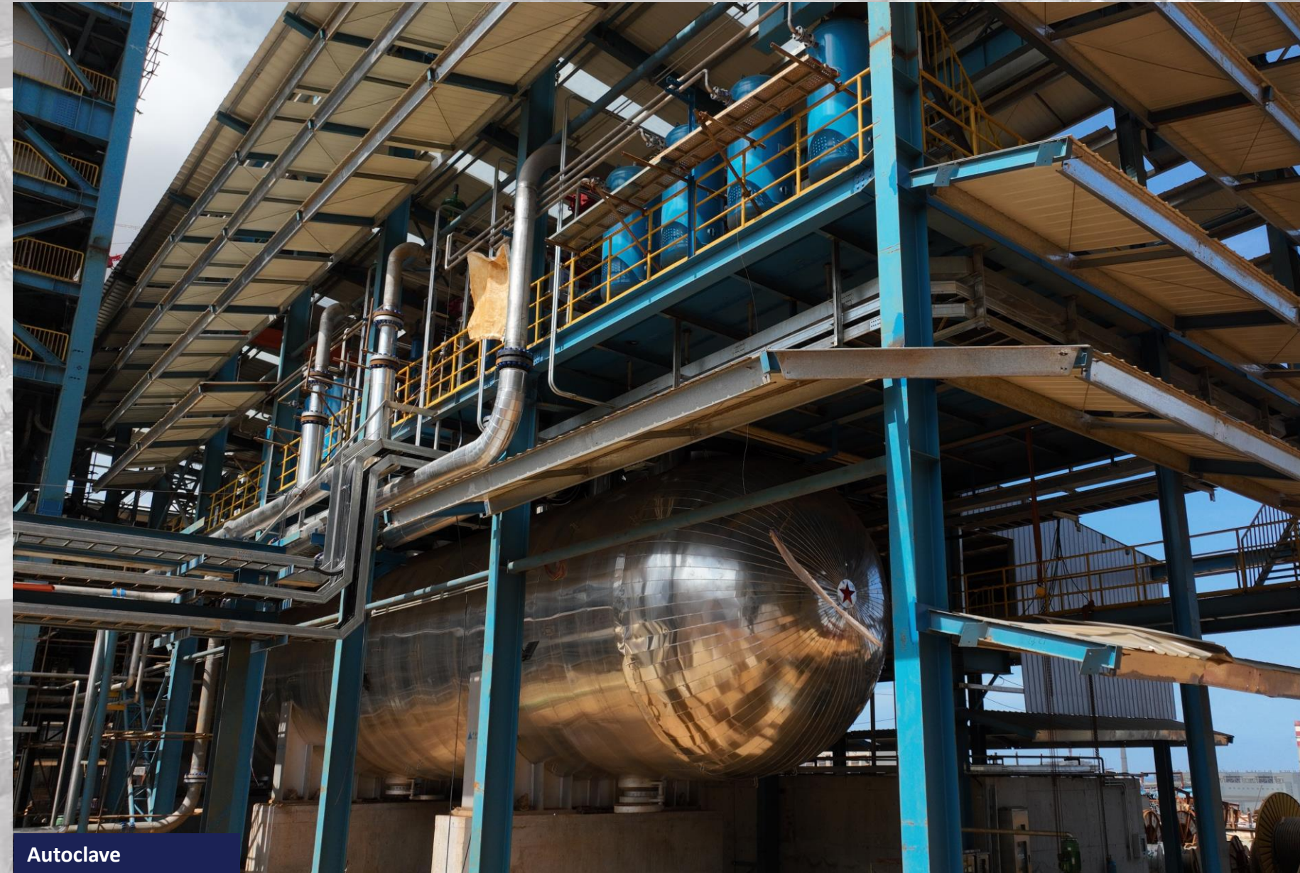
1 st 2 nd and 3 rd autoclave, 1 st 2 nd and 3 rd ore slurry storage & thickening and concentrated sulfuric acid storage tanks
